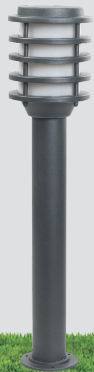
SS 222560 L:Ø16 cm H: 70cm Shape/Style : E27 Arm. Glass : Pleksi Material : Aluminium Paint : Electrostatice
